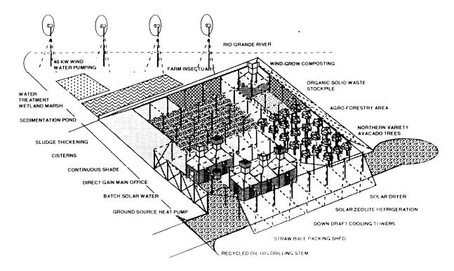
Figure 1: Blueprint Demonstration Farm at Laredo, Texas as Proposed by the Center for Maximum Potential Building Systems.
